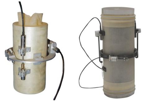
Fig. 6 Hall Effect and LVDT transducer
