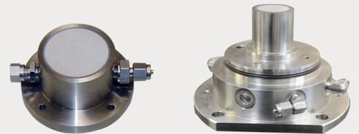
Fig. 7 show an UNSAT pedestal (left) used for Methods A & C and a HKUST pedestal used in method B.
