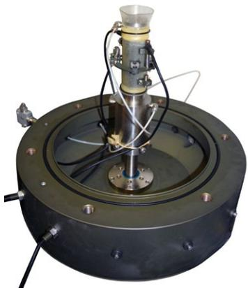
Fig 1. Shows the setup of local strain transducers (LVDT's mounted onto a specimen), as can be seen the cables for the LVDT's pass through the access ring, which allow the transducers to be situated inside the cell without the need for internal connections.
