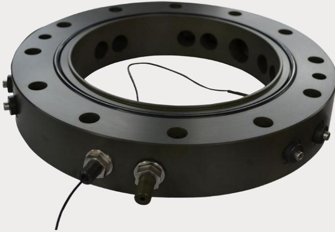
**Overview:** The access rings allows up to 12 transducers / port connections to be added to any of the standard triaxial cell. The access ring sits in between the cell top and the cell base. Extension screws in the triaxial cell, allow the base of the cell to be secured to the top of the access ring.
